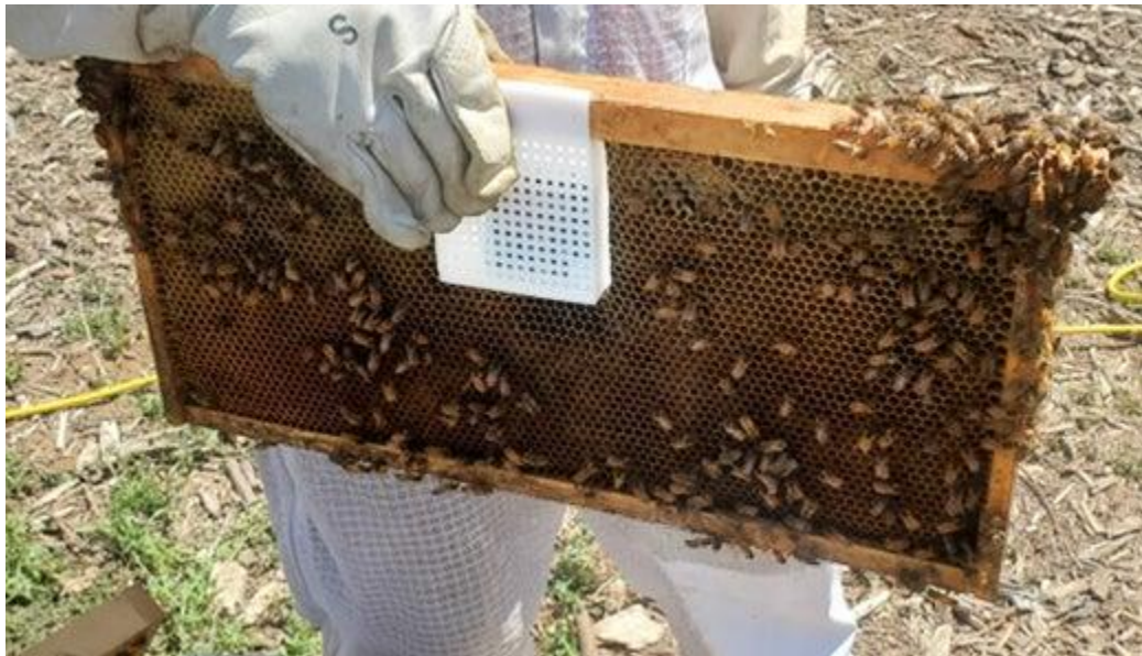
A low-cost heat sensor on a beehive frame (UCR photo)
